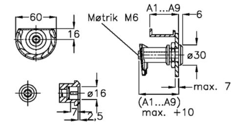
Door + frame thickness = 37-45Measure type = A5
